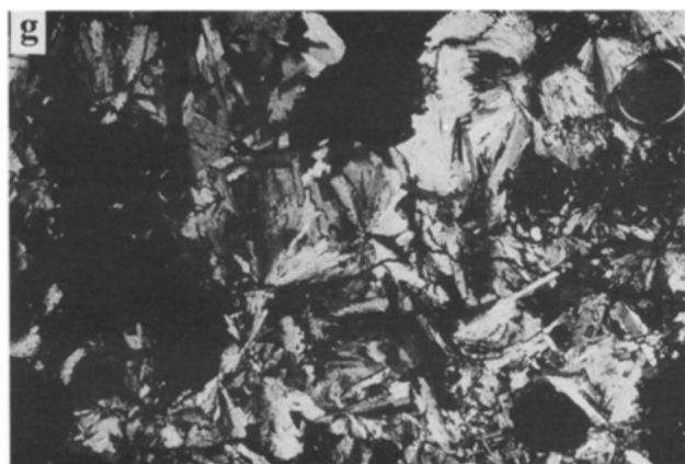
FIG. 8. Continued. (g) Spherulitic devitrification texture of glass between strongly annealed relic grains (relics of mafic precursor minerals are clusters of opaque phases) (sample I-29, 3.4 mm wide, crossed polars).
